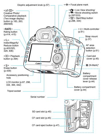
\* Used for wireless connections with the NFC function.
