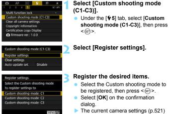
The current camera settings (p.521) will be registered under the Mode Dial's C\* position.
