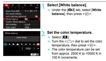
When setting the color temperature for an artificial light source, set white balance correction (magenta or green) as necessary.
