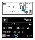
The GPS acquisition status is indicated by the [GC3] icon displayed on the camera's LCD panel.
